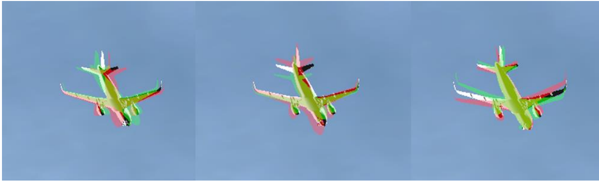
Figure 9: Attitude Error \pm 10^\circ visualized (red/green), Heading (left), Pitch (middle), Roll (right)
