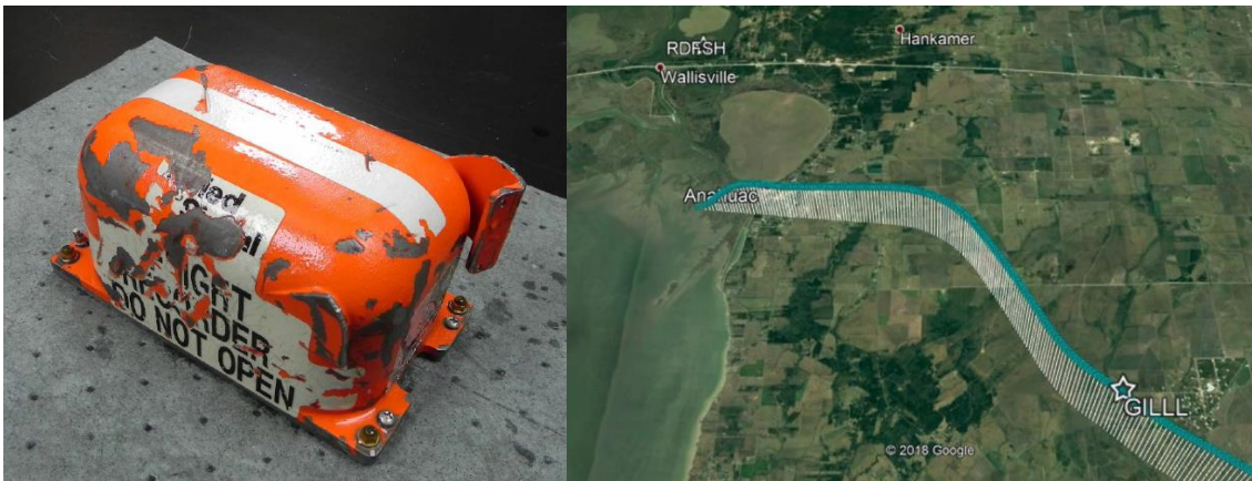
Figure 12: Recovered blackbox (left) and ADS-B flight path data (right) [3]
